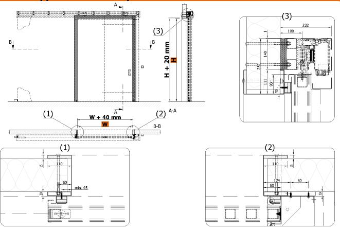
Construction readiness of the opening is secured by the customer according to the requirements of the contractor. It is necessary to respect the flatness of the wall and the floor with a tolerance of max. 3 mm/m.
